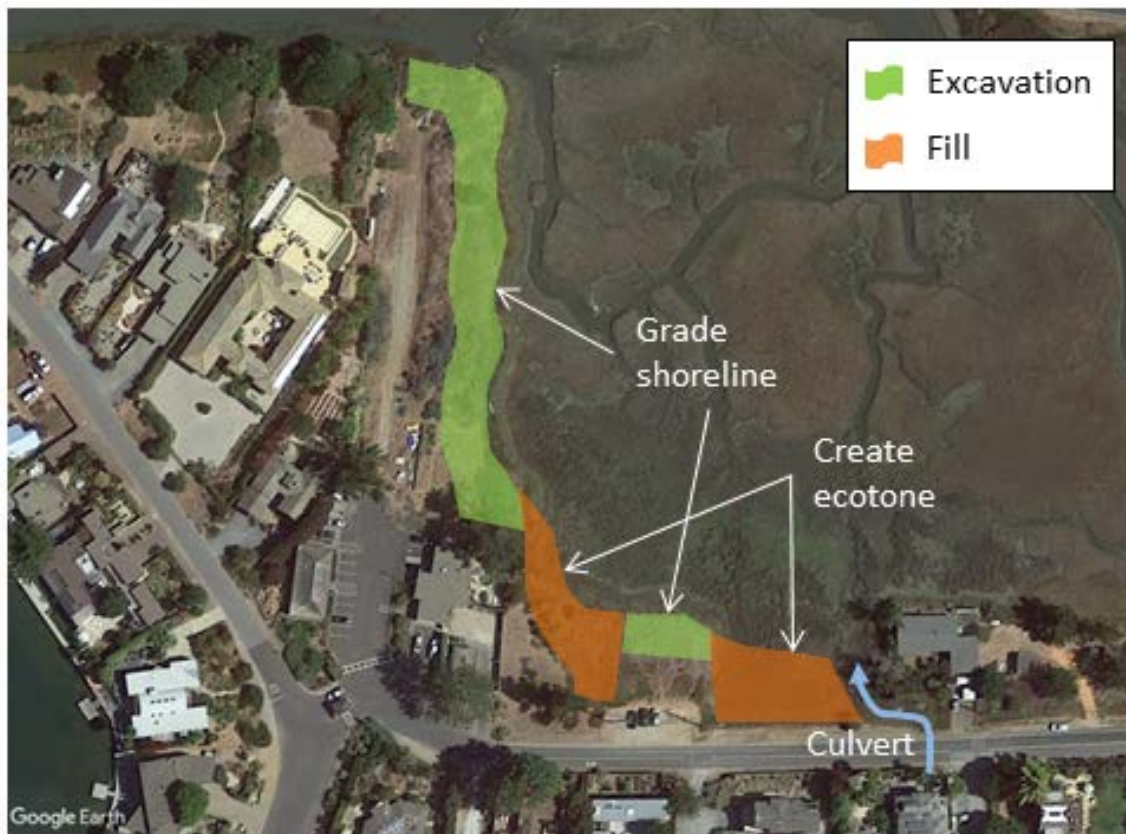
Figure 9. Approximate locations of excavation and fill placement to create transitional ecotone slope
